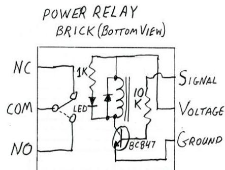
**Figure 8: Bottom View of the Relay Circuit**
